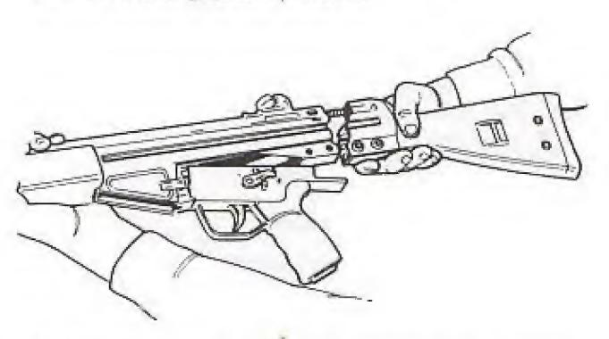
4. Slide the buttstock back into place over the rear of the receiver, with the driving spring properly positioned in its recess in the bolt carrier.
